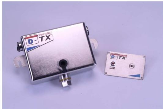
It will detect water contamination triggering an audio-visual alarm at the helm. This allows the operator to drain off the water via the units' drain plug before it enters the engine, before it stops the engine and before it disables the vessel.
